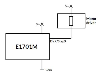
Here "DirX/StepX" symbolises one of the step- or direction outputs, V+ is either V (5V internal, non-insulated mode with both jumpers set) or  $V_{\text{ext}}$  (up to 24V external, insulated mode with both jumpers removed). GND is either GND (non-insulated mode) or  $\text{GND}_{\text{ext}}$  (insulated mode). The internal resistor of the connected device is not allowed to have less than 490 Ohms in order to not exceed the given current limits.
