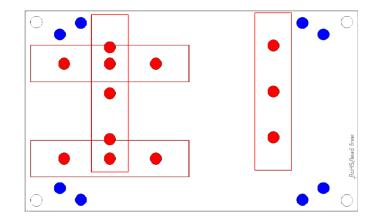
**RED** – mounting positions for DIN/C45 rail locks/DIN/C45 rail adapters (bottom side). Pairs of locks can be mounted in one of 2 possible orientations. Here locks of type Phoenix Contact 1201578 or similar can be used. With these locks the board then can be clamped on a DIN/C45 rail.
